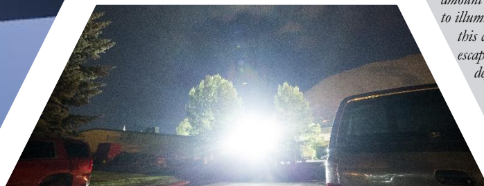
< Fig. 1. An unshielded light fixture (top) as compared to a shielded one (bottom). In a typical unshielded light fixture, 50% of the light produced is wasted. This portion illuminates the surrounding air instead of its intended target on the ground.
